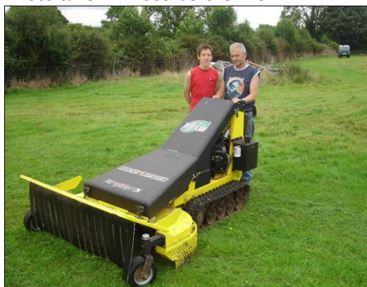
Heather strimming machine used by Gun Club
